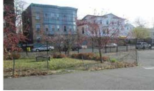
The site is the Paterson Museum located at 2 Market Street. The site appears to have relatively little slope except for a slight slope of the road where each side slopes to the center of the parking lot. The main parking lot has many potholes, and the pavement is in poor condition. It is recommended that it be repaved with pervious pavement. The building has many downspouts that discharge to a lawn which can support a rain garden.
