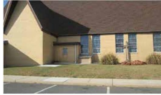
The site is St. Gerard Elementary School located at 16 Carrelton Drive. The site slopes from northwest to southeast. The parking lot in between the school and church is freshly paved. The school has no external downspouts. On the north side of the church is a downspout that drains to grass; a rain garden can be installed beneath it. There is a downspout on the south side of the building as well that could connect to a rain garden.
