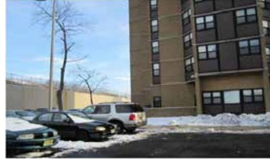
The site is the Governor Residential Apartments located at 27 State Street. The site has a slope from the southwest to northeast. There is also a slight slope north. There are islands in the parking lot that can be converted into bioswales. The sidewalk slopes directly into the parking lot; a rain garden can be placed next to it to divert rainwater from the impervious surface. There is also a courtyard in the center of the complex in which a rain garden or a bioswale can be installed.
